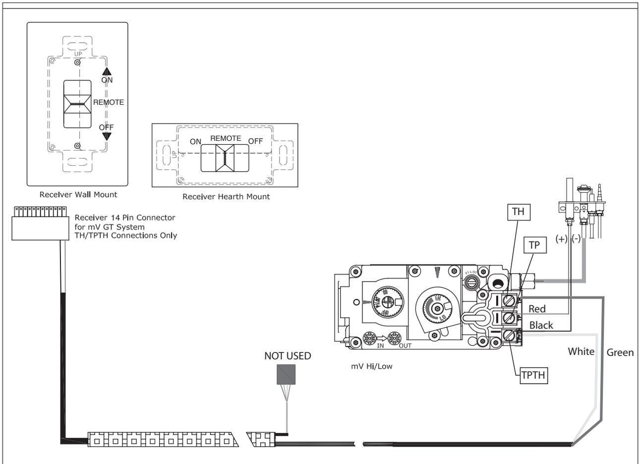
Fig. 5: Connection diagram.
